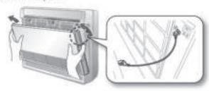
Grab the handle and slightly press the air filter down to bent the air filter. Then, pull the Air filter towards you and lift it up to remove the Air filter.
