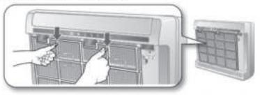
Clean the Air filter with a vacuum cleaner or soft brush. If dust is too heavy, then rinse it with running water and dry it in a ventilated area.
