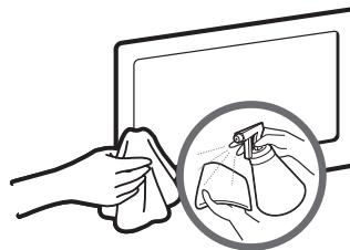
Turn off the TV, and then gently wipe away smudges and fingerprints on the screen with a micro-fiber cloth. Clean the body of the TV with a soft cloth dampened with a small amount of water. Do not use flammable liquids (benzene, thinners, etc.) or a cleaning agent. For stubborn smudges, spray a small amount of screen cleaner on the cloth.
