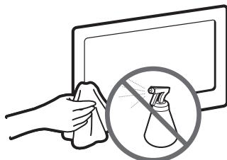
Do not spray water or any liquid directly onto the TV. Any liquid that goes into the product may cause a failure, fire, or electric shock.
