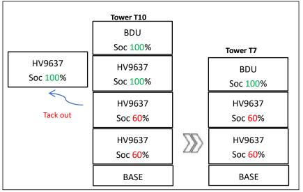
◆ Discharge the original system SOC to between 90~99%. Then continue charging until the inverter shows SOC 100%
