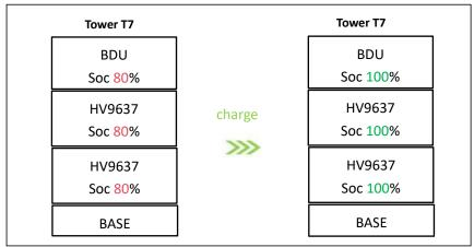
◆ Install the new module with the BDU&Base and use a DC charger to charge the new module. There is a sound of relay disconnection in the BDU, or the charging current is 0, indicating that the battery SOC = 100%.
