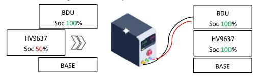
Constant current charging parameter setting: Charging voltage 108V
