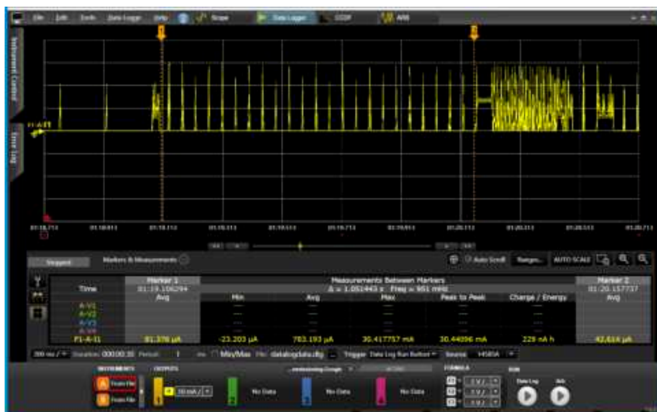
Figure 10.4: BLE connection interval average current @ 45ms
