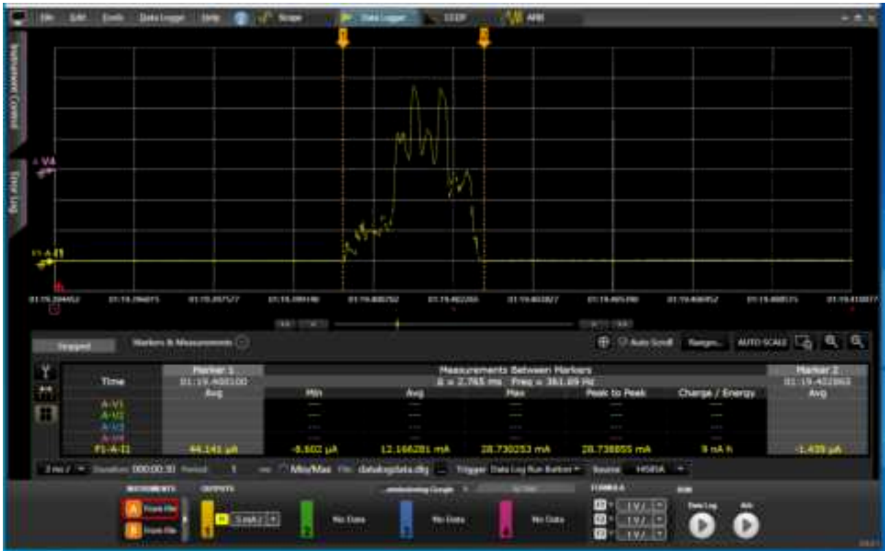
Figure 10.5: BLE connection interval 1 peak current @ 45ms
