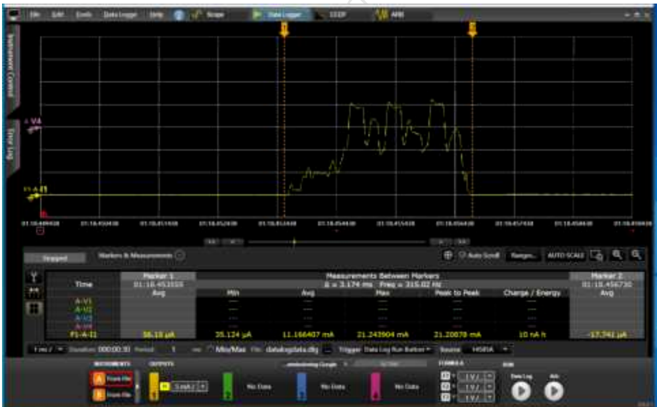
Figure 10.3: BLE advertising active current waveform
