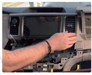
2 Connect the wires between the air conditioning control panel and the original car, and reinstall it back into the original position. Install the bottom plate of the gear lever.
