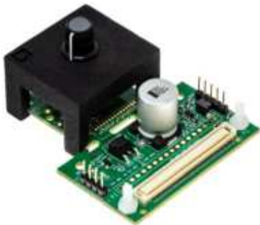
Figure 2. Hardware Configuration Showing the Demonstration Magnet Assembly and the EVAL-ADMT4000SD1Z
