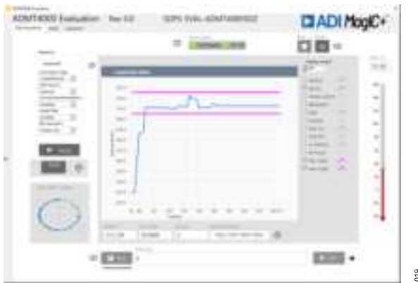
Figure 19. Captured Data Display Showing the Acquired Angle (Blue) and the Target Maximum and Minimum Angle (Magenta) for the Magnetic Reset
