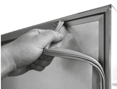
The door gaskets should be cleaned regularly. In case of damage, the replacement of the gaskets is required for the proper operation of the machine. To remove the gasket from the socket, unclasp the corner and slowly pull it out. You can place the new one by pressing it into the sockets.
