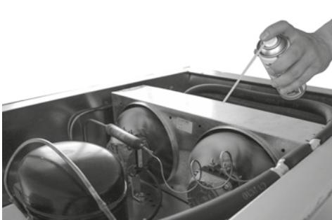
At the upright refrigerators, the condenser area is on the top or below part of the cabinet (depending on the models).
