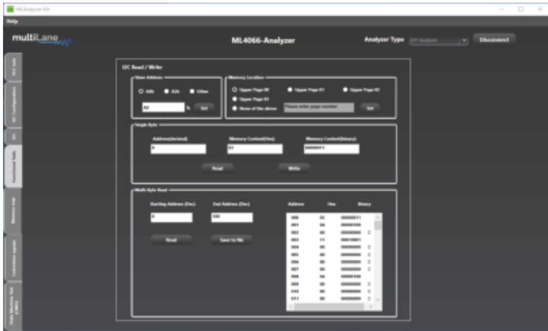
Figure 14: Reading Specific Registers from Functional Tests Tab
