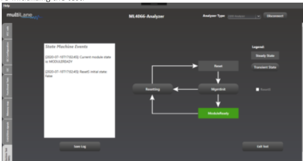
Figure 21: State Machine Test for Flat Memory Modules
