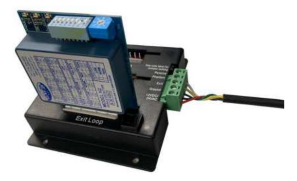
The harness contains a reverse loop, phantom loop, and exit loop. You will need a separate loop detector for each loop.
