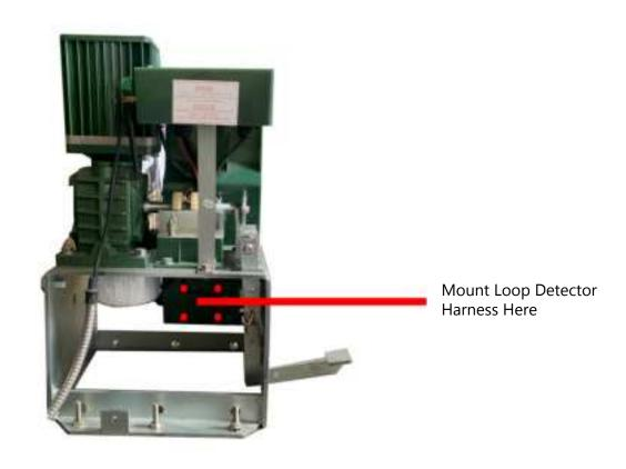
Move the cable from the loop detector harness up into the circuit board compartment, there will be a small circular hole large enough for the cable to go through. Connect the wires based on the wiring diagram in the previous page.
