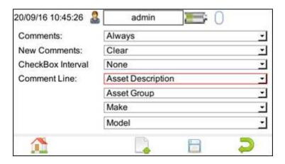
Note: For the four text /comment lines on the Apollo 500 must match the four text / comment lines on PATGuard 3.
