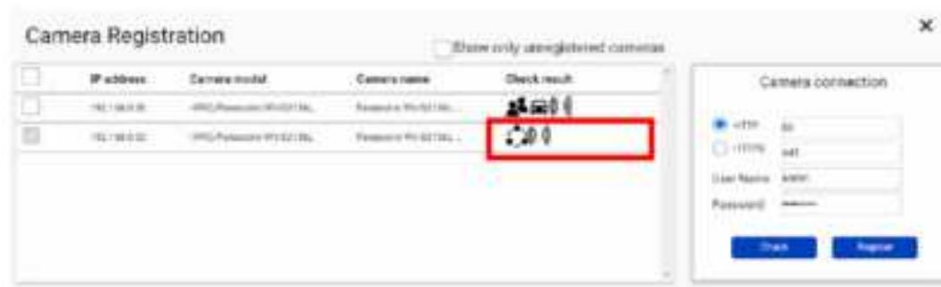
When the 3<sup>rd</sup> party extension software is installed in the selected camera, icon will be shown in the [Check result]. If not shown, please check if configuration file is edited correctly.
