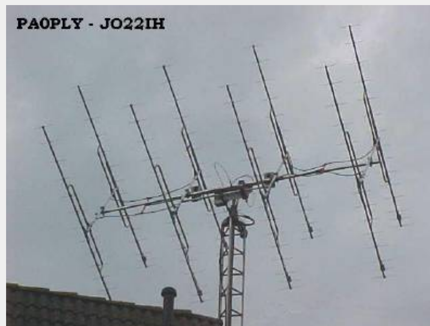
Photo 1.: Large EME array for 432MHz.
