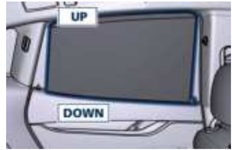
A. Sunshade fully unrolled ("UP" position) and Window closed ("UP" position)
