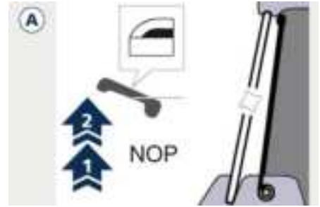
A. Sunshade fully unrolled ("UP" position) and Window closed ("UP" position)
