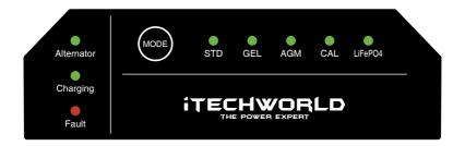
To modify the battery charging profile, disconnect the black (auxiliary) Anderson plug and press the MODE button for 1.5 seconds. The battery type indicator will move one LED to the right.
