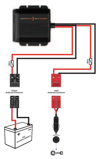
**Output (black Anderson):** connects to the battery being charged (the auxiliary battery).
