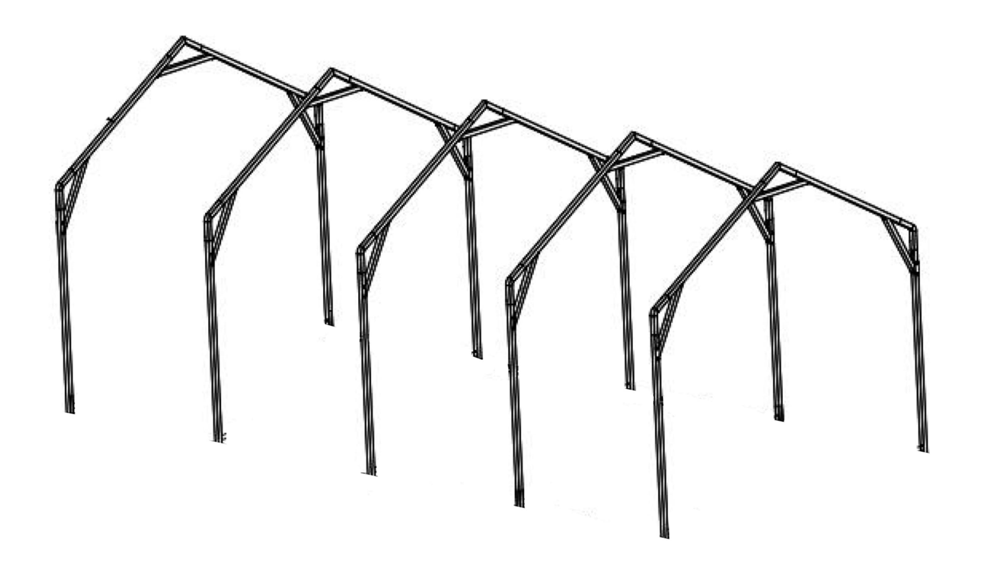
Step 6: Arrange components #A, #J, #I, #I, and #A from left to right as shown, and secure them using self-tapping screws (#4).
