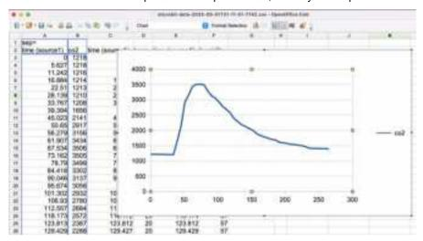
Because the three readings are actually logged at slightly different times, there will be a separate time column, in the CSV file, for each reading type. When creating a chart, just pick one of the time columns for the x-axis – it doesn't matter which.
