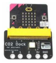
Note that the ring connectors at the bottome of the CO2 Dock are connected to the ring connectors of the micro:bit, allowing you to attach other things to your micro:bit.
