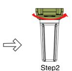
Hold the cup still and turn the base anti-clockwise until it is tightened.
