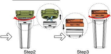
Hold the cup still and turn the base clockwise until loosens
