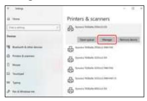
3. Select **Printer properties** from the **Manage your device** list. The Printer Driver Properties window appears.
