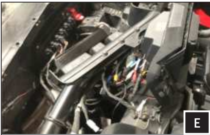
E. Route the MR1 Power Harness into the dash. Route the ring terminal end of the MR1 harness to the bus bar. Cut off the ring terminals and strip the wires.
