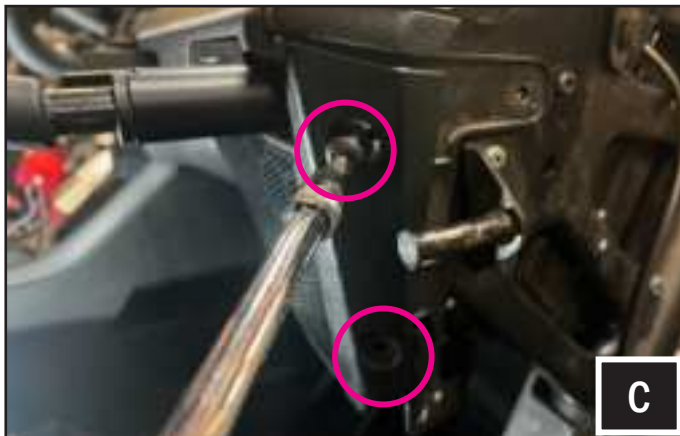
C. Remove the factory speaker grill by removing the (2) screws on the side.
