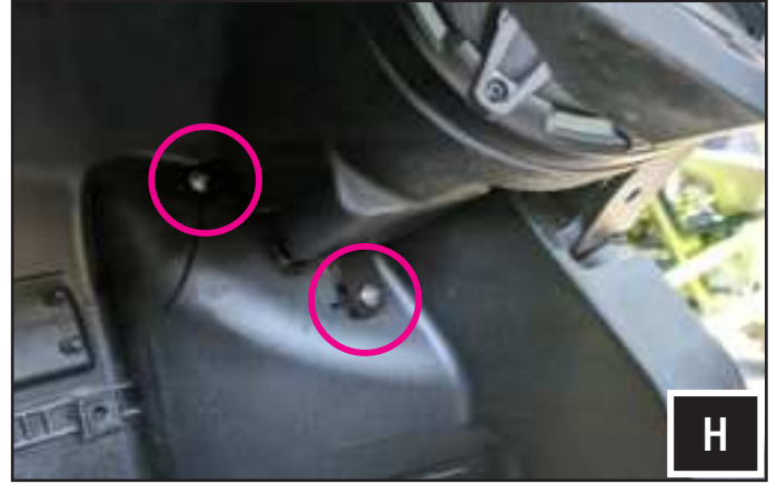
H. Secure the T brackets of each pod to the factory bosses on the footwell using (2 each) #14x.75 phillips screws [B-HP#14-4].
