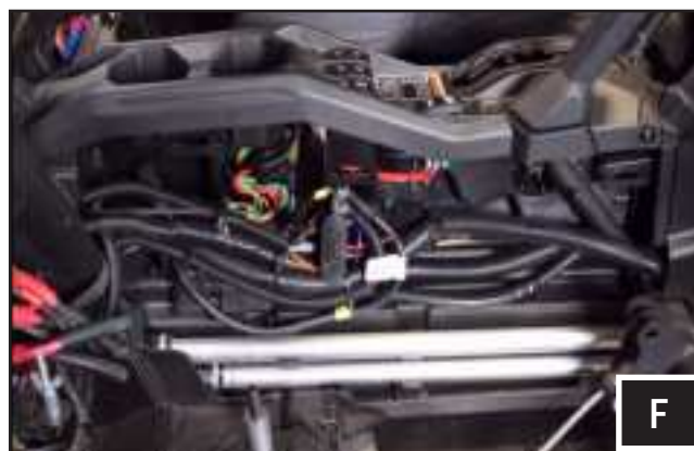
F. Route the speaker extension harness along the center console towards the front of the vehicle. Use zip ties to keep the harness away from any moving parts and any sharp metal. Connect the harness to the JVC to SSV harness adapter (B-H2367).
