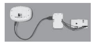
In case of Network Installation with online management, the thermostat and the Control Card must be paired with a Network Programmer specific to the property before the installation.
