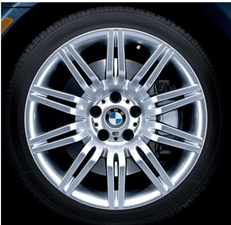
□ 19 x 8.5 front, 19 x 9.5 rear Double Spoke (Style 172M) cast alloy wheels with 245/35R-19 front, 275/30R-19 rear performance tires. 1 (incl. in 550i Sport Package; spare is a space-saver wheel and tire)
