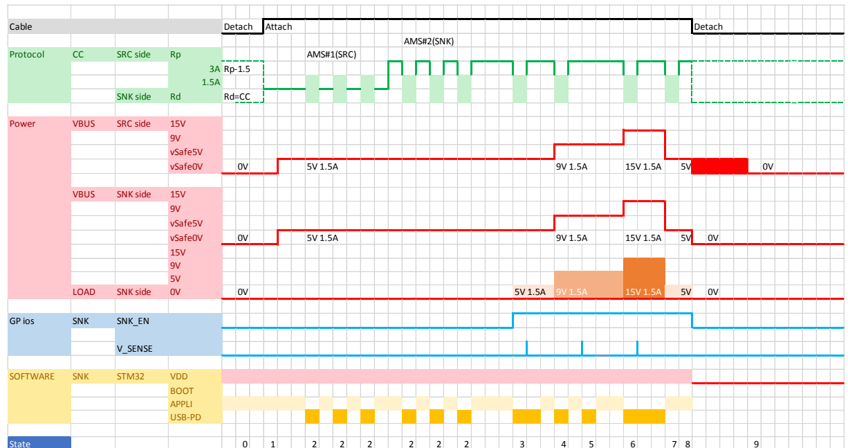
Figure 23. Sink external power time line
