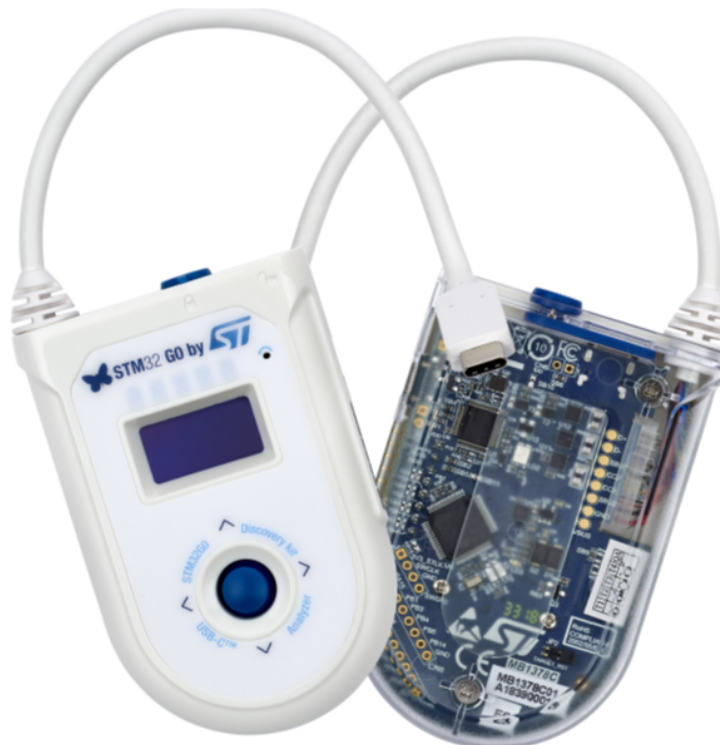
Figure 9. STM32G0 Discovery kit USB Type-C analyser
