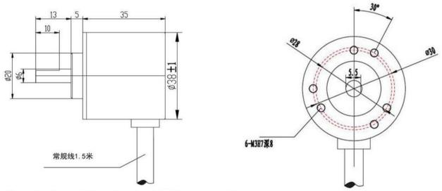
Dimensions in mm. Unless otherwise stated, tolerance: ±0.5mm
