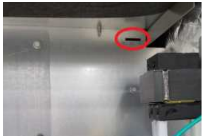
FIGURE 18. Notch for Control Panel Relocation
