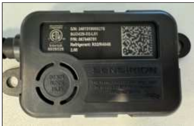
FIGURE 22. Example of Clear, Unobstructed Sensor Inlet
