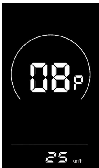
Figure 6-9 Speed limit setting interface
