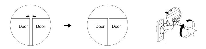
If the gap is too tight between the two doors, loosen the screw at the front of the hinge as shown to make the adjustment and then re-tighten the screw.
