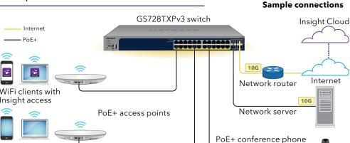
. Connect devices to the RJ-45 ports (depending on the model, 1-24 or 1-48) on the switch front panel.
