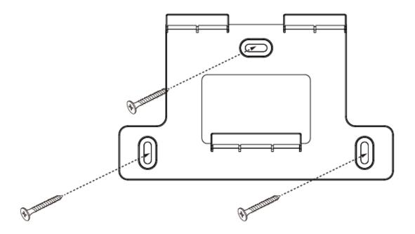
**Step 4.** Attach the Touchscreen Keypad onto the bracket.
