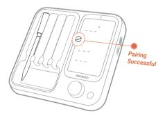
3.Follow the app instructions, put the new, unpaird probe in the charging position of the base, and start charging. The app will show the pairing interface, while the display area of the corresponding number on the device will show the pairing icon " " Wait for the device to pair automatically, and you can use the probe after the device tells you that the pairing is successful
