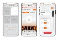
1. Open the application, click on the corresponding number to enter the probe page, then go to the settings to remove the probe and confirm.
