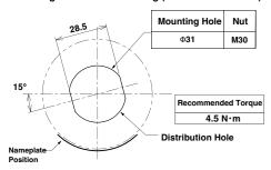
■ W4/W5/W8 Direct Mounting (Mounting with M30 Nut) / M12 Connector
