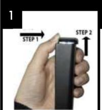
Looking at the keypad, slide the dark lens cover away from you (STEP 1) and lift the lid from the back (STEP 2).
