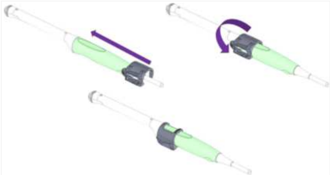
BK 8819 and E10C4 Probe Holder mounting instructions
