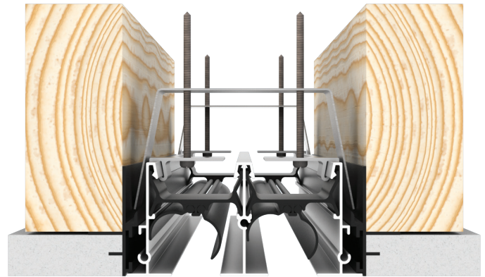
Figure 15 (Step 5B): Install Linear Into Sub Frame
