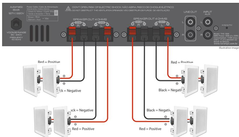
For this kind of connection use cables with a minimum gauge of 1.5mm<sup>2</sup> for up to 40 meters. For long distances, consult the table on page 12 "Important recommendations". It's necessary to make connections in parallel and series as shown in the example, to match impedance.
