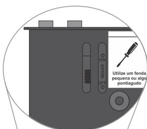
To enable, disconnect the device from the socket and place the switch located at the bottom in the ON position. Use a small screwdriver or something similar.
