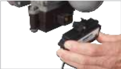
2. Press the activation module onto the sensor.
