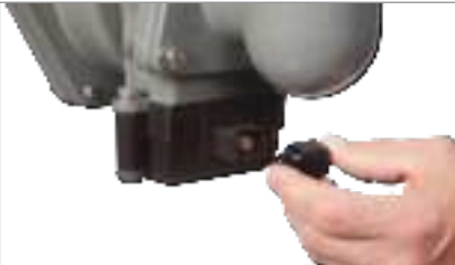
1. Remove the dust cover from the sensor.
