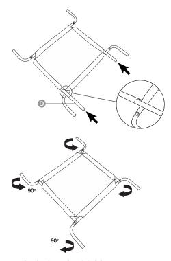
Insert the two metal bars into the mat through the holes.
