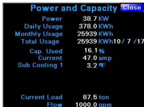
Figure 19. Power and capacity control screen
