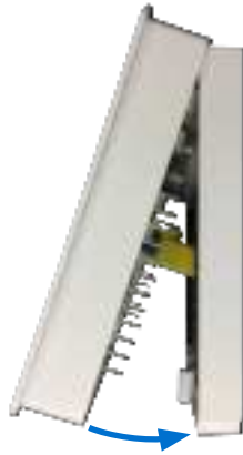
Illustration 7—Reinstalling the Cover on the Backplate
