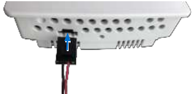
Illustration 14—MS/TP (EIA-485) Data Port
