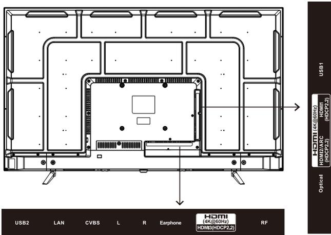
**USB:** Connect the USB device such as the flash disk to access the TV media function.
