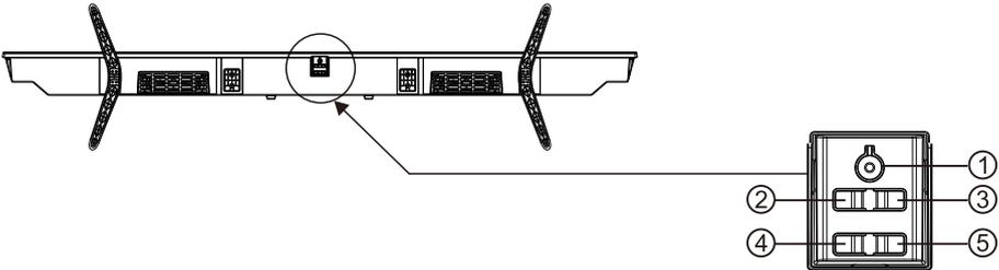
1. **⏻/MENU**: When TV power off, short press this button to turn on. When TV is on, long press this button to turn off, short press this button to call out the TV menu, press the VOL+/- and CH+/- button to select the menu and press the power on/off button again to confirm the selection.
