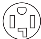
4-wire receptacle (14-30R)
