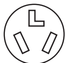
3-wire receptacle (10-30R)
