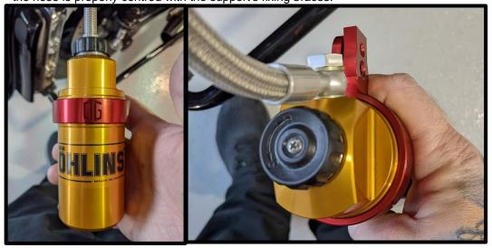
b. **Legend suspension:** Place the reservoir support on the reservoir using the provided Legend reservoir shim. Refer to the pictures below for alignement reference.
