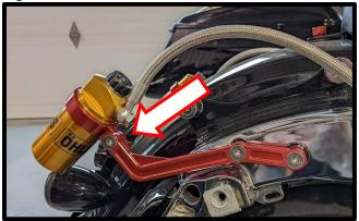
b. **Legend suspension:** Install the reservoir mount on the support arm on both side using the 5/16"-18 flat head screw supplied with the kit. Make sure the hose is routed as shown on the picture. Secure the hose as shown in the picture below with the supplied zip tie.
