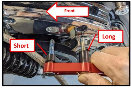
9.B) ) Install the support arm on each side of the motorcycle and make sure the spacers are positioned as shown in the picture below.
