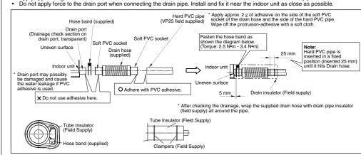
(3) Insulating the Drain Hose Selection of heat insulation materials for drain hose (Drain insulator). When using the heat insulation materials (field supply), kindly use
