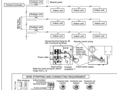
te: lating Devices (Disconnecting means) should have minimum 3.0 mm contact gap
