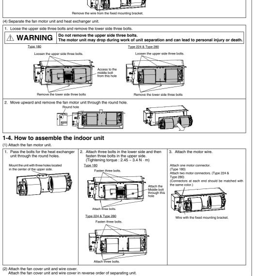
2. Move the fan cover unit upward and remove it through the round hole
