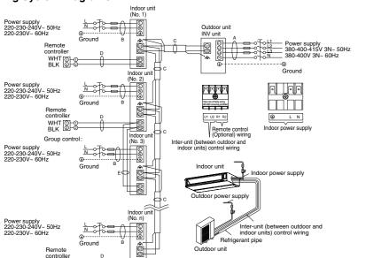
1) See the section "3-3. Recommended Wire Length and Wire Diameter for Power Supply System" for explanation of "A", "B", "C", "D", and "E" in the above diagram (2) The basic connection diagram of the indoor unit shows the 6P terminal board, so
