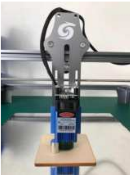
Place the 20mm fixed column on the surface of the carved object
