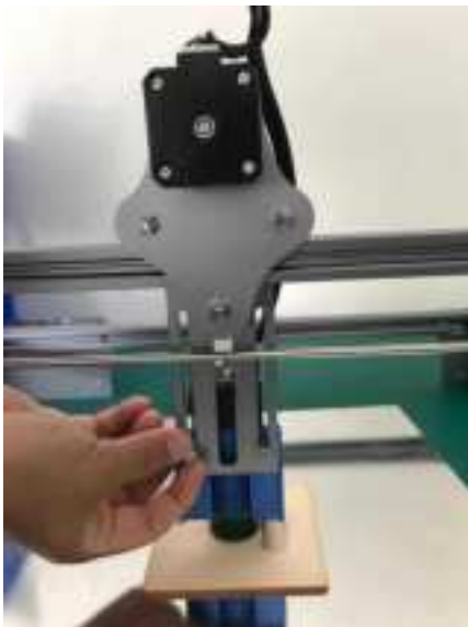
Tighten the fixing screws, And remove the fixed focus column
