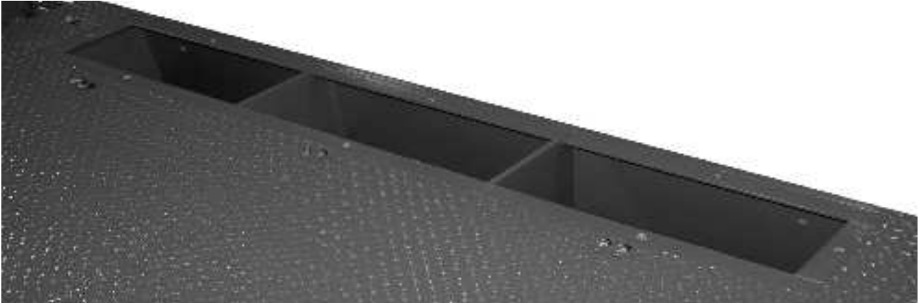
Figure 5-2. End Cleanouts with bolts and cover plate removed
