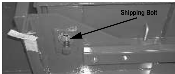
Figure 2-5. Weighbridge Shipping Bolts
