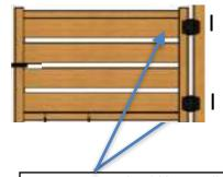
Hinges position should be installed as shown in drawing [2.5 inches from the top and bottom]
