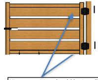
Hinges position should be installed as shown in drawing [2.5 inches from the top and bottom]
