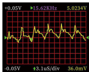
High-speed voltage ripple (AC coupling)
