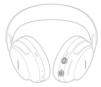
The status light blinks white. After 30 seconds, the status light blinks amber to indicate factory settings are being restored (2 to 3 seconds).
